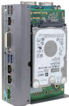
▲ POC-300 with MezIO® - R11 and 2.5" HDD
