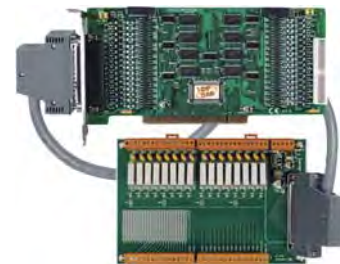
PISO-P32C32 with DB-16P16R: 16-ch input terminal and 16-ch Relay (3A, Form A) board, 1 m cable.
