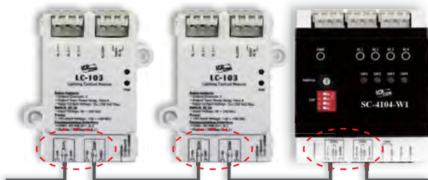
RS-485 and Power Input Daisy Chain using an RJ-11 Connector
