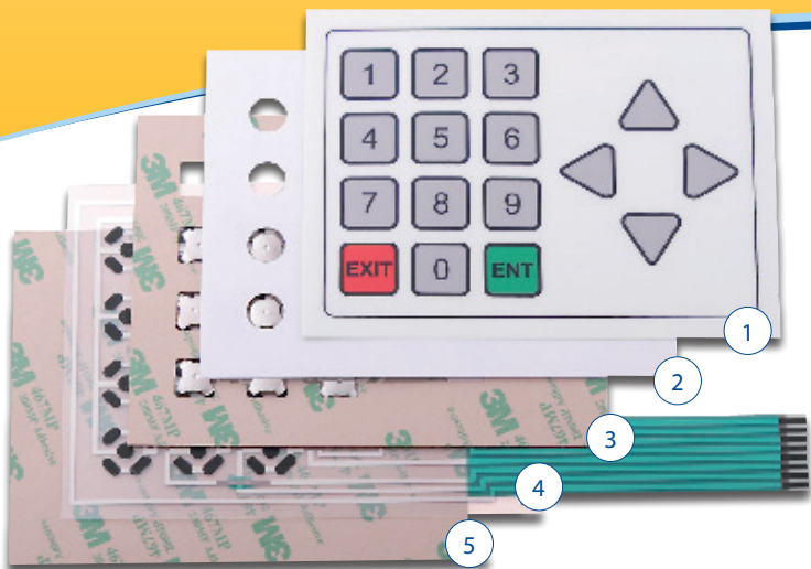
Layer construction of a flexible membrane keyboard 1 PCB track foil with integrated switching elements (switching foil) 2 Spacer foil 3 Retaining/ protective foil (optional) 4 Adhesive foil for design foil 5 Design foil
