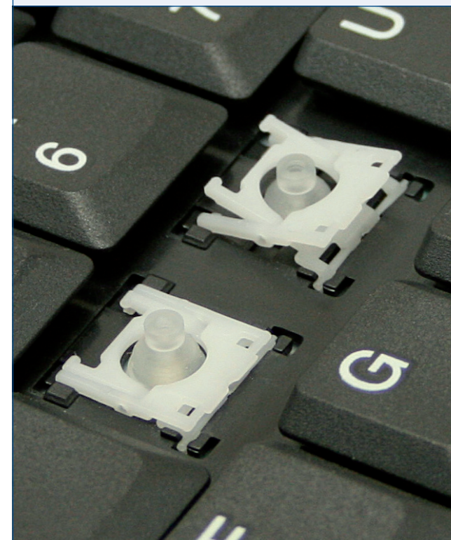
Long Travel Keys with Scissors Technology
