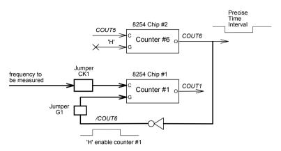
Figure 4.5 Example of frequency measurement (1)
