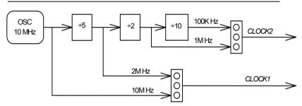
Figure 2.4 Clock system of ACL-8454
