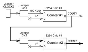
Figure 4.3 Example of frequency generator (2)
