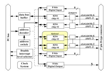
Figure 1.1. Block diagram of the ACL-8454
