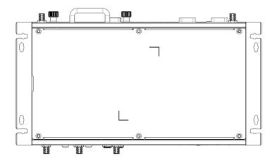
2. Insert full size WWAN module in marked place.
