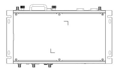
2. Remove 2.5" drive bay and Insert half size WLAN module in marked place.
