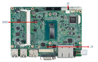
Figure 3.1 Top side of main board
