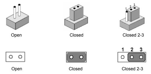
A pair of needle-nose pliers may be helpful when working with jumpers. If there are any doubts about the best hardware configuration for the application, contact the local distributor or sales representative before making any changes.
