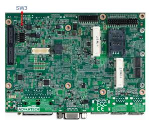
Figure 3.2 Bottom side of main board
