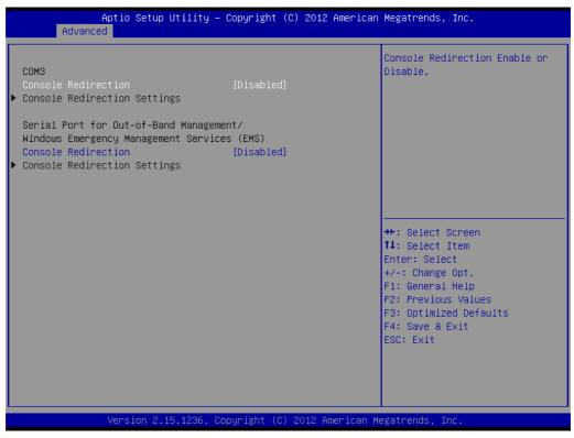
Figure 5.17 Serial Port Console Redirection
