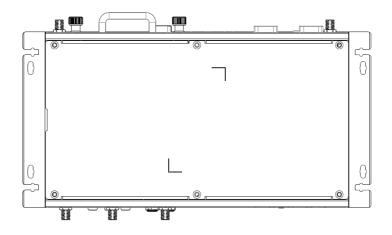
2. Remove 2.5" drive bay and Insert full size mSATA storage in marked place.
