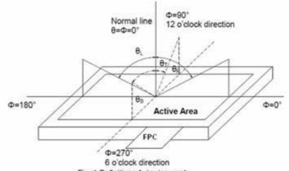
Fig. 1 Definition of viewing angle
