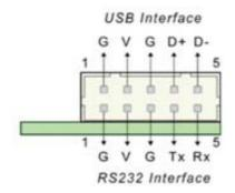
Figure 6.1 Board mounted header
