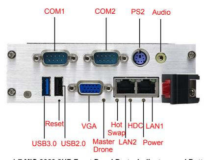
Figure 1.7 MIC-3329 8HP Front Panel Ports, Indicators and Buttons
