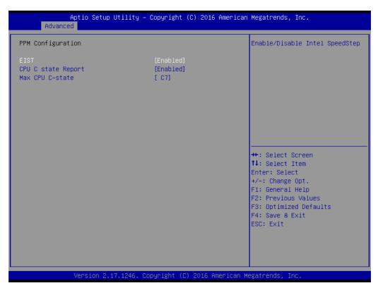
Figure 2.9 PPM configuration
