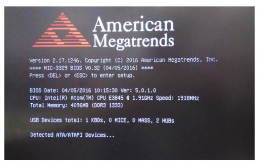
Figure 2.2 Press <DEL> or <F2> to Run Setup
