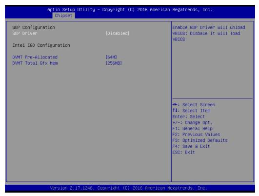
Figure 2.19 Intel IGD configuration
