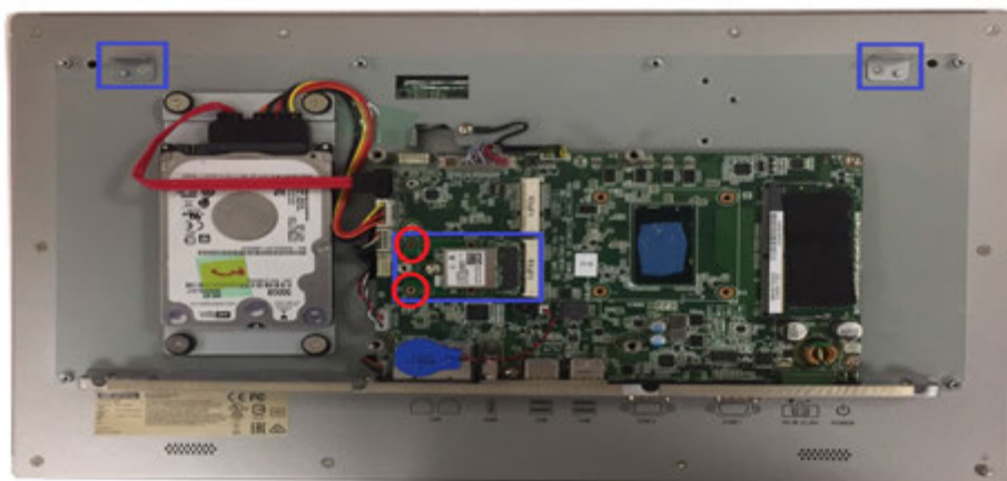
Figure 2.13 Installing the wireless LAN card
