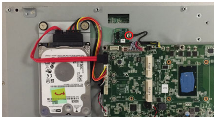
Figure 2.18 Fix TPM card with LVDS cable
