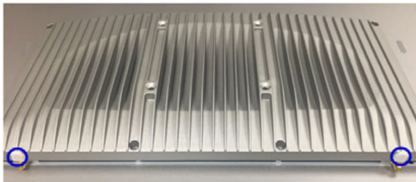
Figure 2.16 Removing plugs for the antennae
