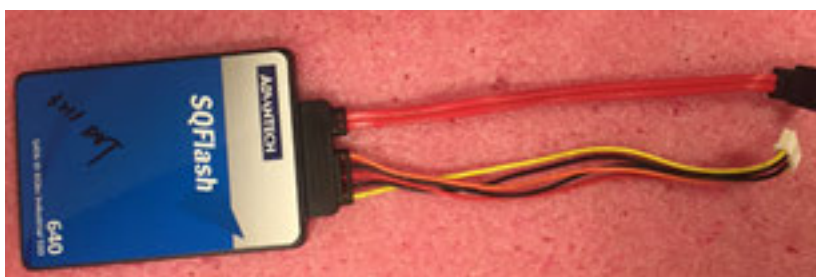
Figure 2.9 SATA cable connected to SATA HDD
