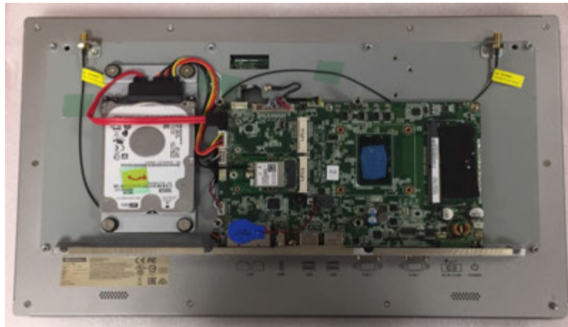
Figure 2.15 Full-size mini PCIe LAN antenna cables
