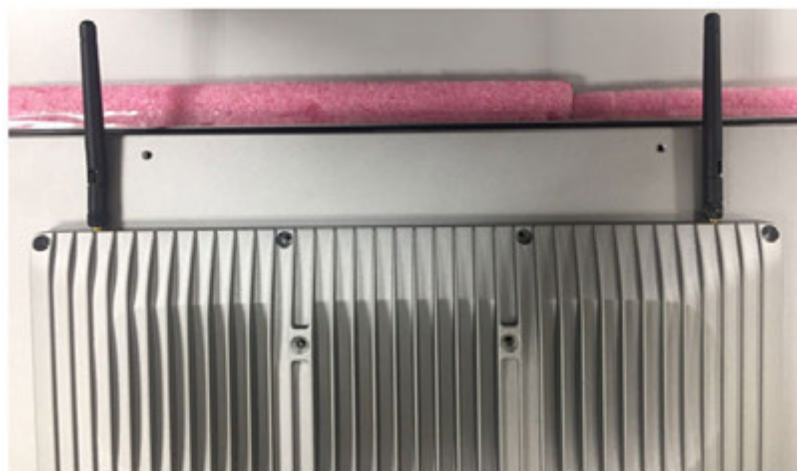
Figure 2.17 Location of external antennae
