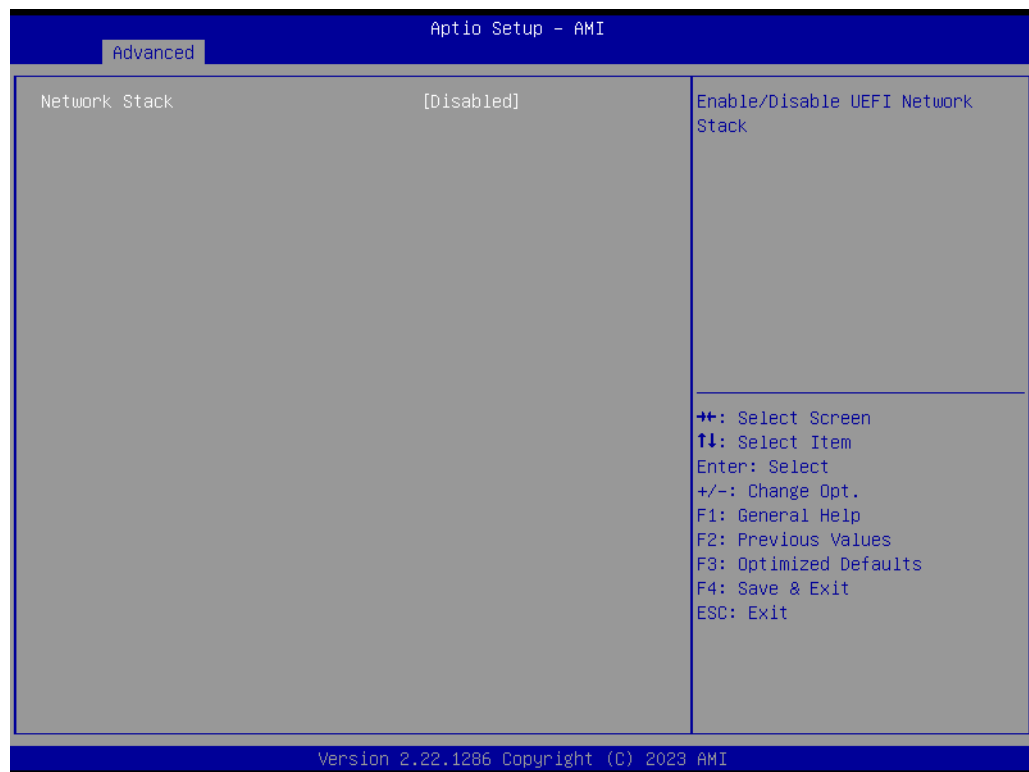
Figure 3.16 PCI Network Stack Configuration
