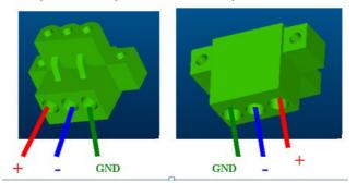
**Figure 2.3 Pin Definition of Power Connector**
