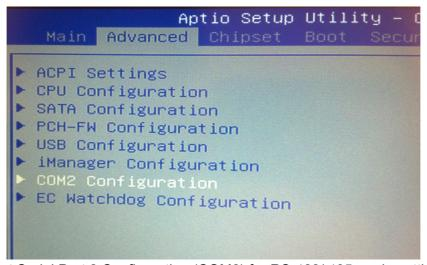
3. Select Serial Port 2 Configuration (COM2) for RS-422/ 485 mode setting.
