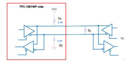
When using RS422/485 port of TPC-1581WP/1881WP, please apply below formula to calculate terminal impedance to meet the standard.  $V_{\it fsb}=0.2V$
