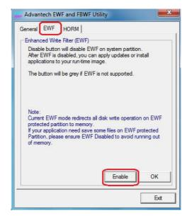
3. After the system is rebooted automatically, EWF enable
