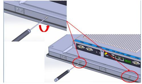
**Step 3**: Set TPC cross the cut-out hole and push it into the wall, the snap hook will hold the machine on the wall.
