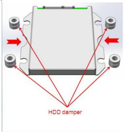
Step 3: Install HDD module into system and then cover back the side cover to finish.
