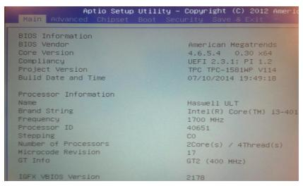
2. Enter into Advanced tab and select Serial ports Configuration.
