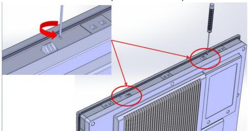
Step 2: And then release the 2 screws in the bottom of TPC
