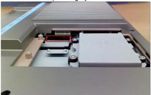
Figure 2.2 Install CFast Memory Card
