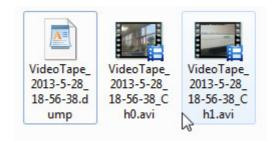
VideoTape\_2013-5-28-18-56-38.dump includes two channels. After the conversion, VideoTape\_2013-5-28-18-56-38\_Ch0.avi and VideoTape\_2013-5-28-18-56-38\_Ch1.avi will be generated automatically. When using the "Dump to vids", it will convert all channels into one "\*.vids" file.
