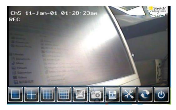
The default storage disk is disk D. The storage disk will be automatically switched to disk E if disk D is out of space (free space should not be less than 2G. When the recording function is enabled, the system will automatically generate the Tape file at D:\. The D:\Tape\stroge.index. is reserved while all video files are stored at D:\Tape\Tape\. For example: D:\Tape\Tape\VideoTape-November-26-2012\_14-47-56.vids. (As shown below.)
