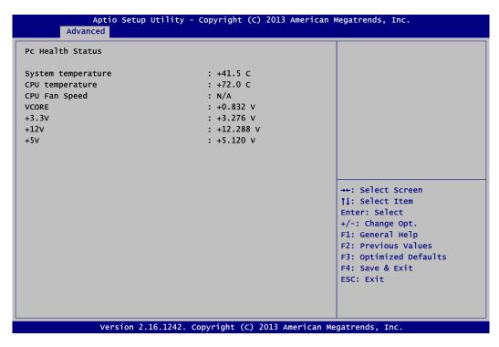
This screen displays the temperature of system and CPU, system voltages (VCORE, +3.3V, +12V and +5V).
