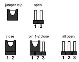
Properly configure jumper settings on the CAPA841/842 to meet your application purpose. Below you can find a summary table of all jumpers and onboard default settings.
