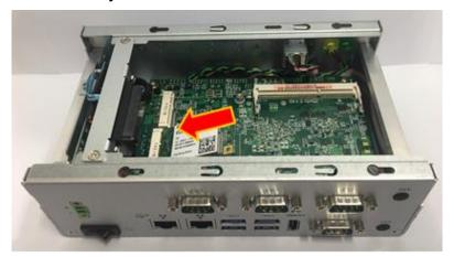
Step 6 Press it down gently, but firmly, and then secure the PCI Express mini card to the carrier by tightening up the one M2\*5L Phillips pan head screw to the marked position.
