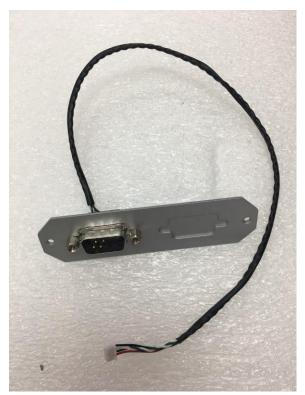
Step 6 Loosen two screws to remove the bracket from the panel.
