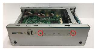
Step 7 Fasten the CAN Bus bracket into the chassis.
