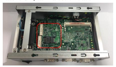
Step 5 Holding the PCI Express mini card at a 45 degree angle up from horizontal, slowly insert the golden fingers into the PCI Express slot until it is fully inserted in.
