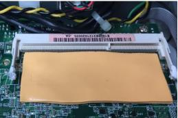
Step 5 Holding the DDR3L SO-DIMM at a 30 degree angle up from horizontal, slowly insert the golden fingers into the DDR3L SO-DIMM slot until it is fully inserted in.
