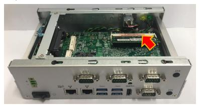
Step 6 Press it down gently, until it is firmly seated by locking two latches on the sides.
