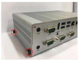
Step 3 Pull out the HDD/SSD drive bay bracket.
