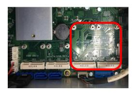
Step 5 Assemble I/O connector with bracket and fix this I/O bracket into the Flexible I/O Window
