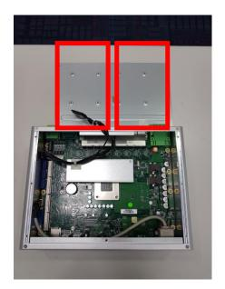
Step 5 Assemble the SSD/HDD with the four HDD mounting screws. Make sure the PCB side of the SSD/HDD will be facing the bottom cover and connected the SATA power cable.
