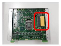
Step 4 Locate the memory module, insert a gold colored contact into the socket and push the module two end latches till locked and put the top DRAM thermal pad from accessory pack onto the top of DRAM.
