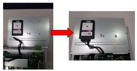
Step 6 Put the bottom cover and fasten all the screws back onto the system.
