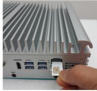
[Note] The system provides two PCIe slots for SIM card installation. Pay attention to the orientation when inserting a SIM card: The SIM card's contacts must face downward when the card is being inserted into the SIM1 slot; the card's contacts must face upward when it is being inserted into the SIM2 slot.
