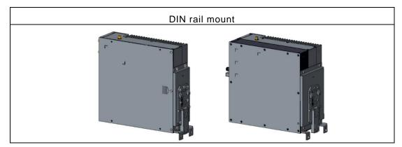
**Step 1** Screws the below two parts together with seven screws.
