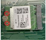
**Step 5** The IPC950 supports three antenna openings, please remove the antenna plugs from the cover and Install the antenna cables, then screw the bracket. Installation completed.
