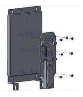
Step 2 Fasten the DIN rail to the chassis with four screws. Installation is complete.
