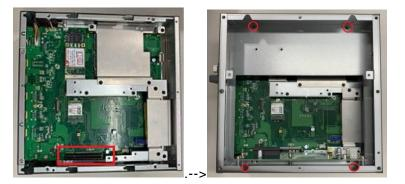
**Step 3** After installing the expansion box kit, close the cover back to the chassis and fasten the screw. Installation is complete.
