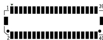
Diagram 2-4 CN2 pin mapping
