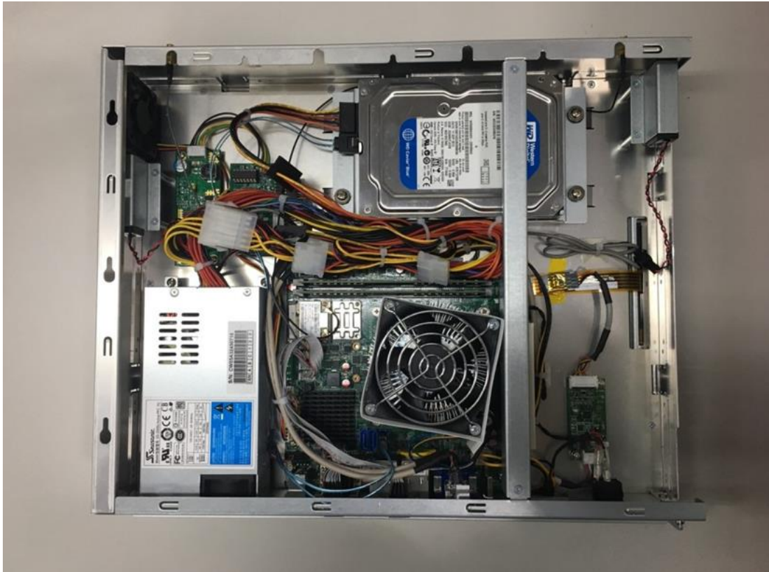
Figure 2-2 After Removing the back cover of the P1177E-500, install memory, storage and any other peripherals.
