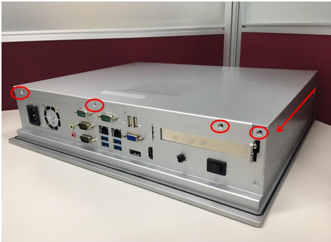
Figure 2-1 Removing the back cover of the P1177E-500
