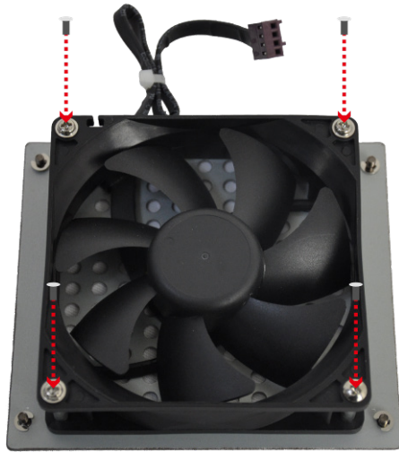
Figure 3-5: System Fan Installation
