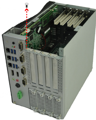
Figure 3-20: Remove Expansion Slot Bracket
