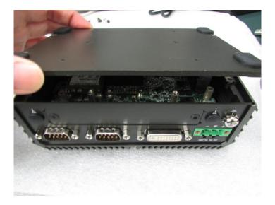
2. Fasten the 4 screws to fix the cover.
