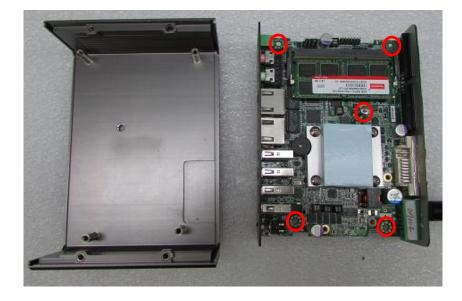
2. Make sure the either sides of front and rear panels are in the chassis grooves and insert the body of unit into Chassis. Use the 3 screws to fasten the body and chassis together.
