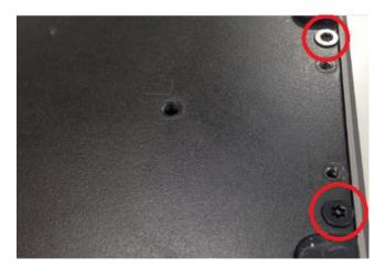
3. Place the side mount bracket on bottom of system as picture below, and fasten the rest of 4 screws to fix it with system together.
