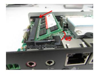
3. Press the module down until it's fixed firmly by the two locking latches on the sides.
