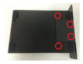
4. Fasten the screws through the bracket mounting hole to mount system on the wall.
