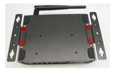
2. Fasten the screws through the bracket mounting hole to mount system on the wall.
