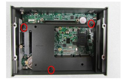
2. Make the PCB side of the HDD face up, place the HDD bracket on it. Ensure the direction of bracket is correct and use 3 provided screws to assemble HDD and HDD bracket together.
