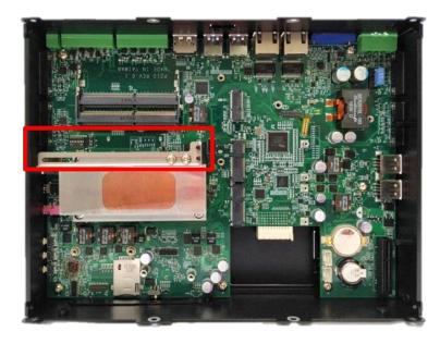
8. Loosen the two screw as indicated to have the clamp arm slidable.
