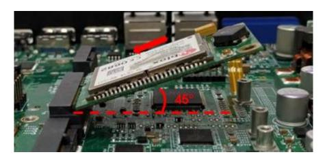
3. Press the card down and secure it with 2 screws.
