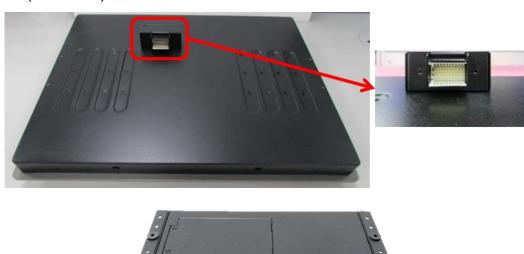
6. Place the P2100 on the display module through its display connector hole as indicated.
