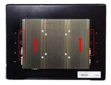
8. Fasten six screws to secure P2100 on the display module.
