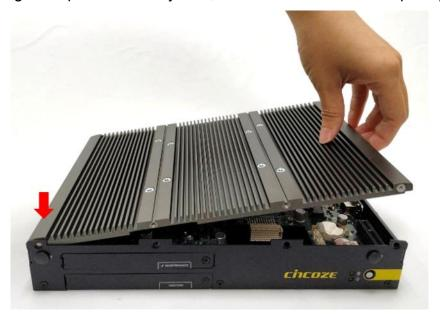
2. Fasten the eight screws at front and rear panel to secure the top cover.
