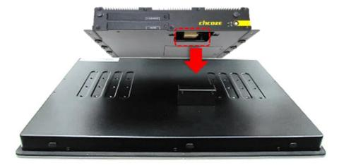
7. Align the mounting holes of P2100 with the screw holes of display module underneath. Then slide the PC2100 carefully as indicated to have P2100 and display module connected together.
