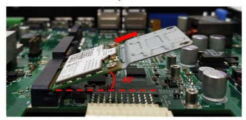
4. Press down the card and secure it with two screws.
