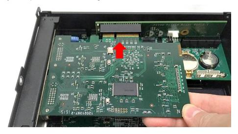
6. Fasten the screw back to secure the PCI(e) expansion card.
