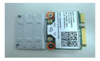
3. Tilt the Mini PCIe card at a 45-degree angle and insert it into the socket until the golden finger connector of the card seated firmly.
