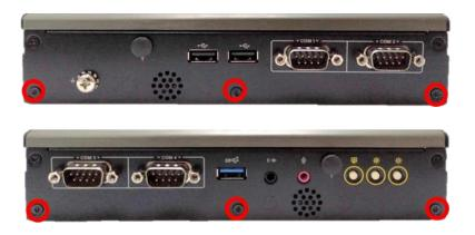
3. Assemble two wall mount brackets by fastening six screws from the screws pack.
