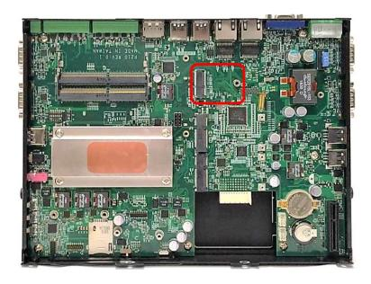
2. Tilt the M.2 E Key card at a 45-degree angle and insert it to the socket until the golden finger connector of the card seated firmly.
