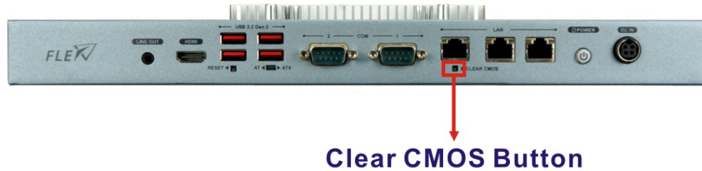
Figure 3-21: Clear CMOS Button Location
