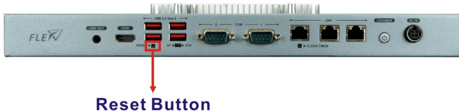
Figure 3-24: Reset Button Location
