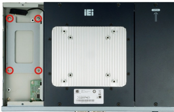
Figure 3-2: HDD Bracket Retention Screws
