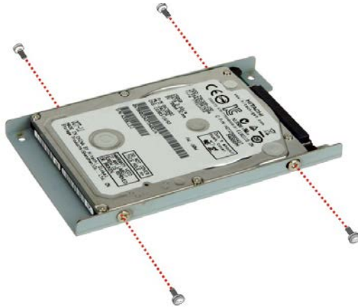
Figure 3-3: HDD Retention Screws
