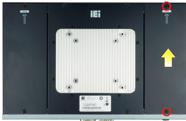
Figure 3-5: PoE Card Cover Retention Screws
