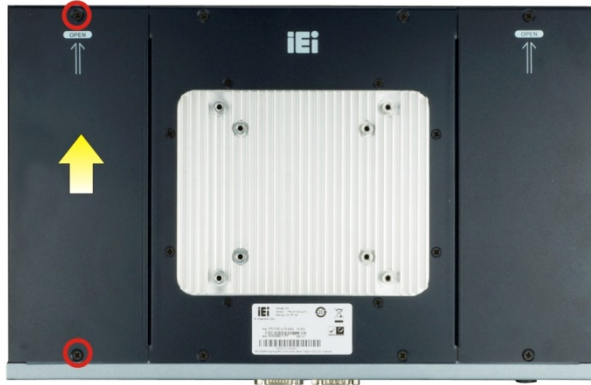
Figure 3-1: HDD Cover Retention Screws
