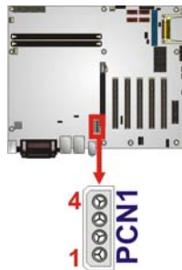
Figure 3-11: PCIe Power Input Connector Location
