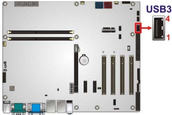
Figure 3-33: USB 2.0 Connector (Type A) Pinout Location
