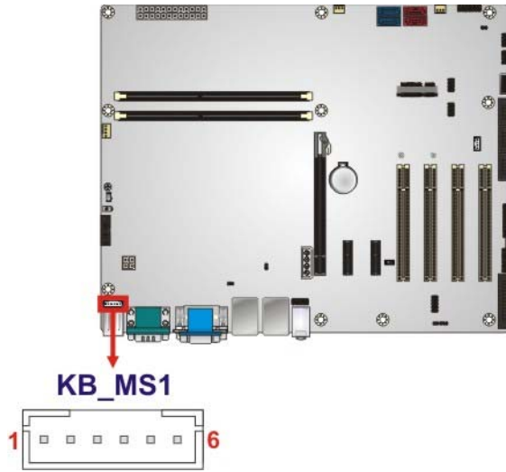
Figure 3-16: Keyboard and Mouse Connector Location
