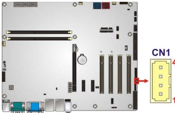
Figure 3-29: SMBus Connector Location
