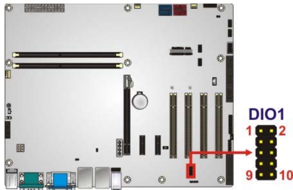
Figure 3-8: Digital I/O Connector Location
