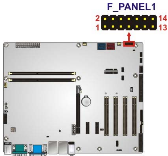
Figure 3-13: Front Panel Connector Location
