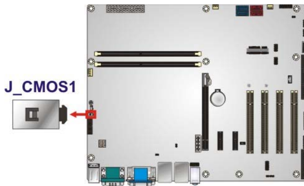
Figure 4-11: Clear CMOS Button Location
