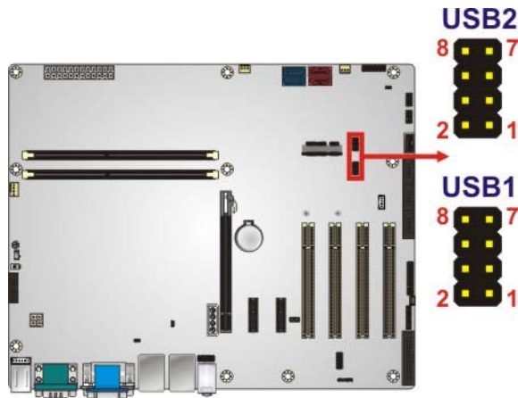
Figure 3-34: USB 2.0 Connector Pinout Locations
