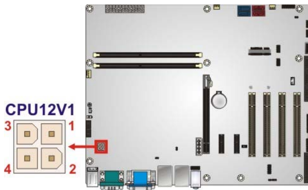
Figure 3-2: +12V Power Connector Pinout Location
