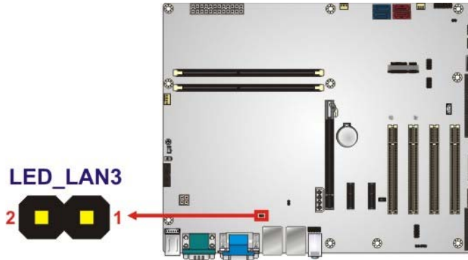
Figure 3-17: LAN1 LED Connector Location
