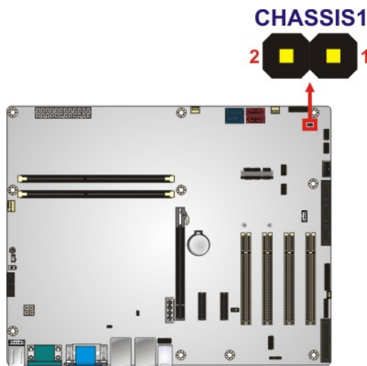
Figure 3-6: Chassis Intrusion Connector Location
