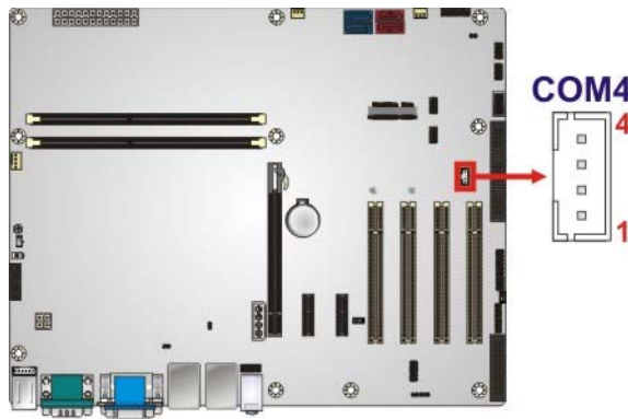
Figure 3-28: RS-422/485 Connector Location
