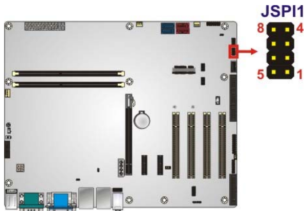
Figure 3-30: SPI Flash Connector Location
