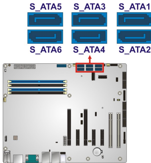
Figure 3-24: SATA 6Gb/s Drive Connector Locations
