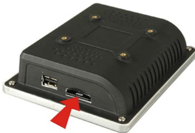
Figure 3-1: Mini SD Card Installation
