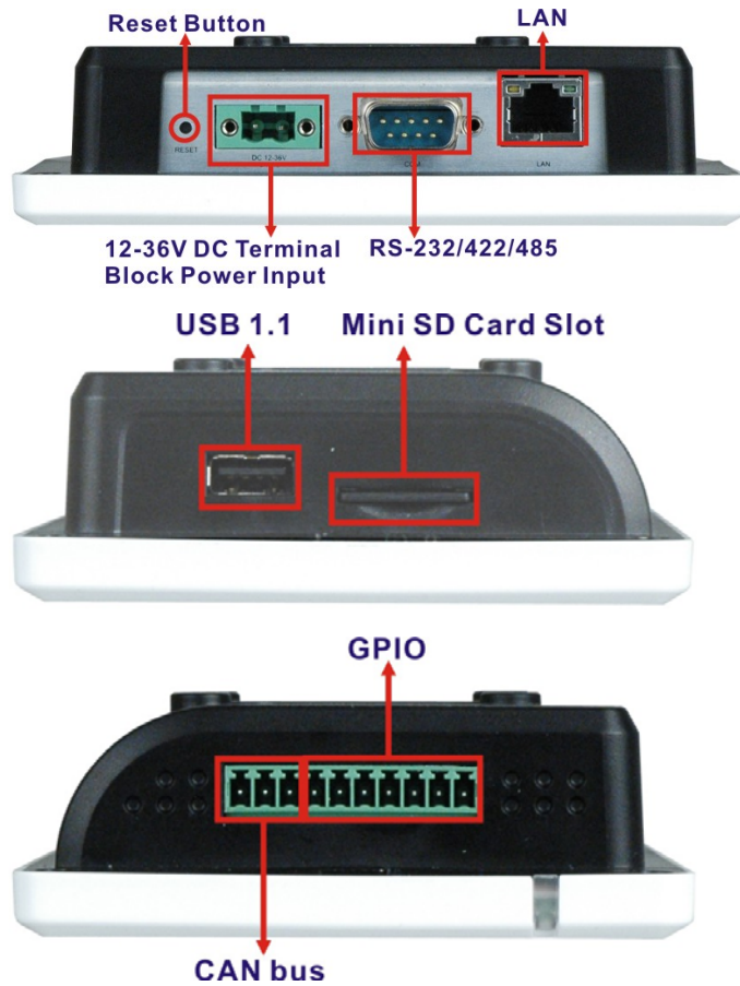
Figure 1-3: IOVU-430M Peripheral Connectors
