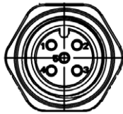
Figure 3-15: Audio Connector Pinout Location
