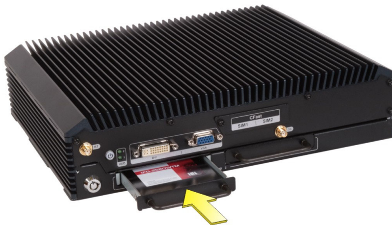
Figure 3-9: Installing the HDD/SSD Tray
