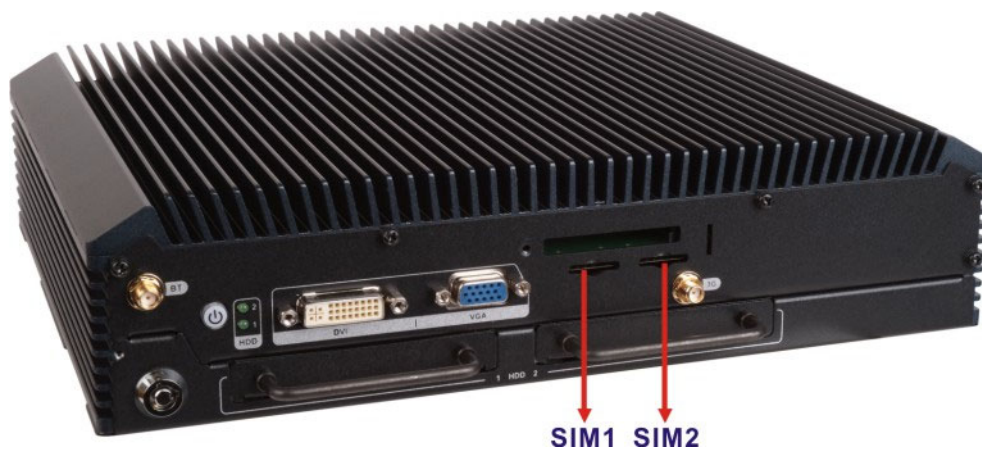
Figure 3-13: SIM Card Slot Locations
