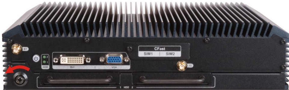
Figure 3-6: Unlocking the HDD/SSD Trays
