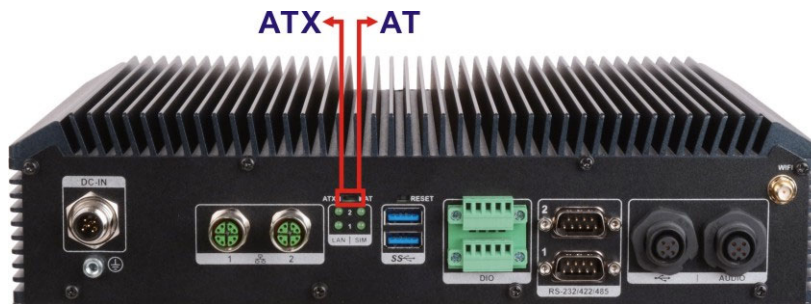
Figure 3-2: AT/ATX Mode Selection Switch Location
