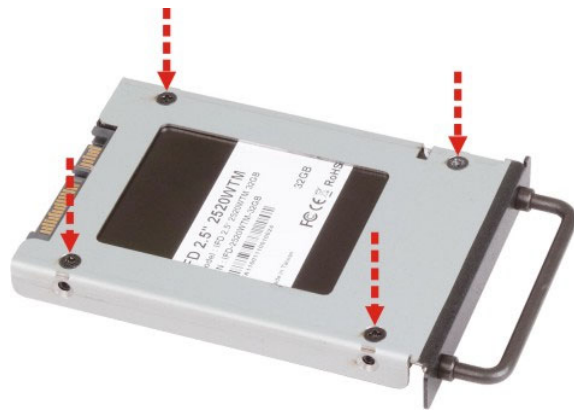
Figure 3-8: HDD/SSD Retention Screws
