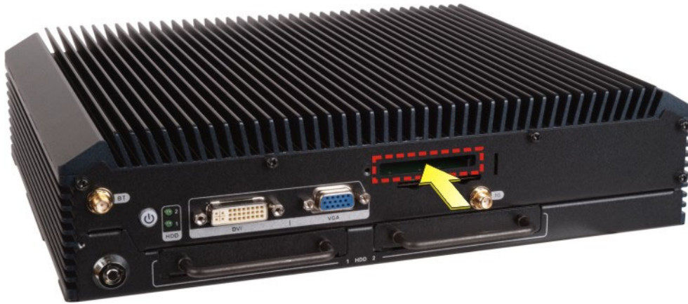
Figure 3-12: CFast Card Installation
