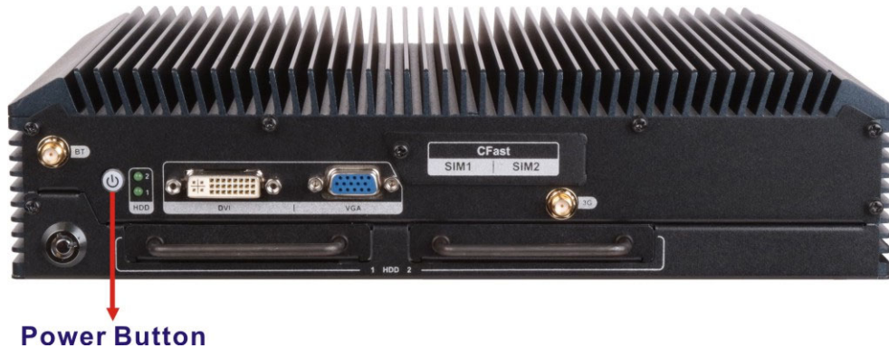
Figure 3-25: Power Button with LED Indication
