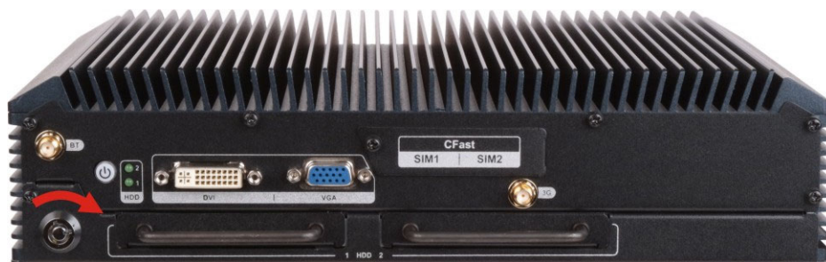
Figure 3-10: Locking the HDD/SSD Trays
