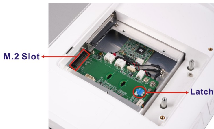
Figure 3-6: M.2 Slot Location
