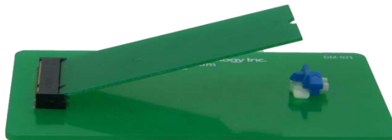
Figure 3-7: Inserting the M.2 Module into the Slot at an Angle
