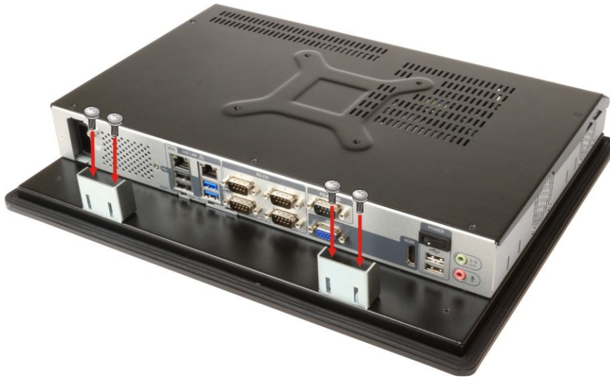
Figure 3-29: PPC-F15A-H81 Mounting Bracket Installation
