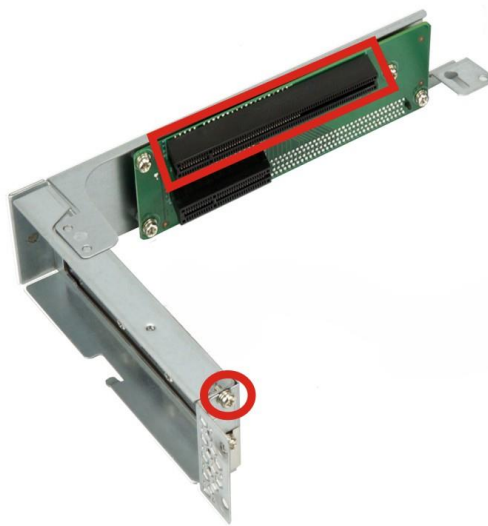
Figure 3-13: Blank Bracket Screw
