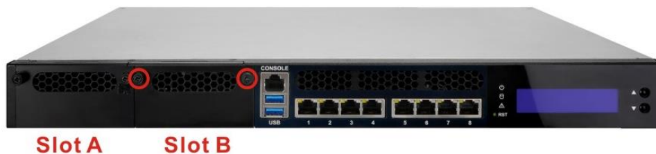
Figure 3-16: Networking Module Slot Cover Screws
