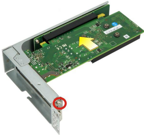
Figure 3-14: PCIe Expansion Card Installation
