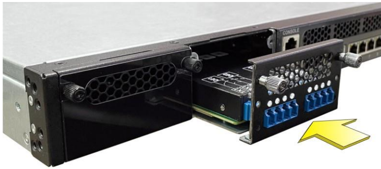
Figure 3-17: Networking Module Installation
