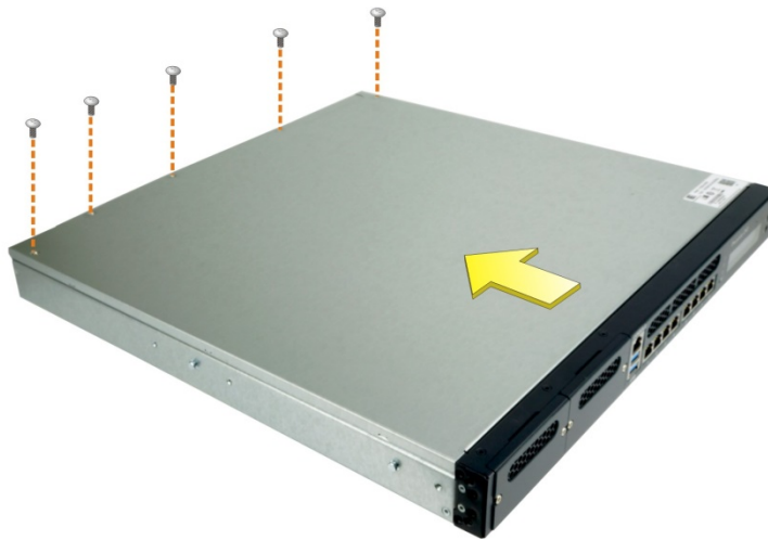
Figure 3-1: Top Cover Removal
