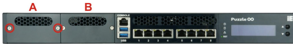
Figure 3-11: Networking Module Slot Cover Screws
