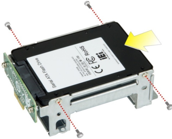
Figure 3-4: Secure HDD to the Bracket
