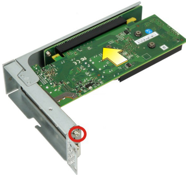
Figure 3-9: PCIe Expansion Card Installation
