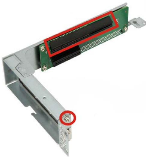
Figure 3-8: Blank Bracket Screw
