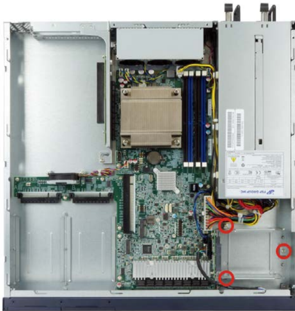
Figure 3-3: HDD Bracket Retention Screws
