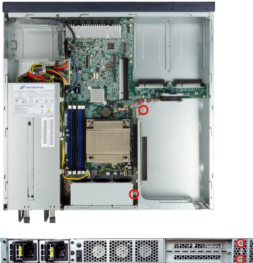
Figure 3-6: Expansion Slot Module Retention Screws
