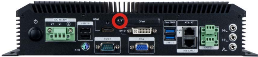
Figure 3-1: CFast Slot Cover Retention Screw
