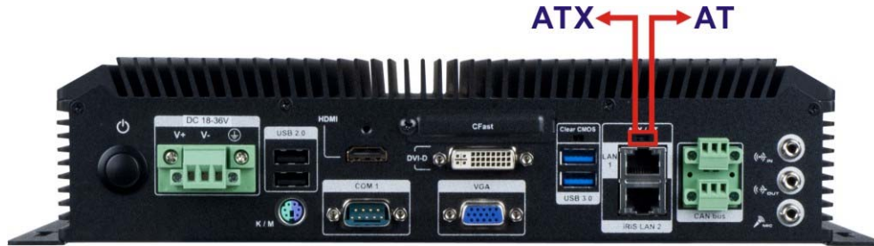
Figure 3-7: AT/ATX Mode Selection
