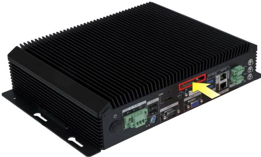
Figure 3-2: CFast Card Installation
