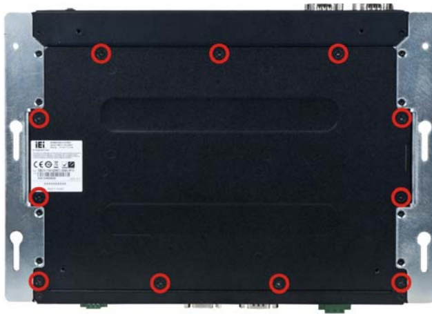
Figure 3-3: Bottom Cover Retention Screws
