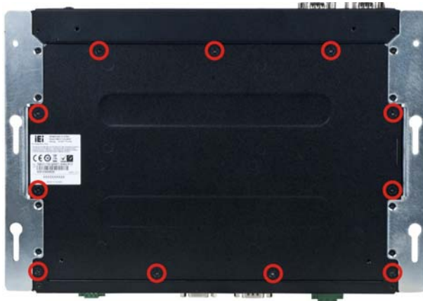
Figure 5-1: Bottom Cover Retention Screws
