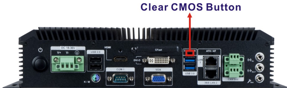
Figure 3-14: Clear CMOS Button Location
