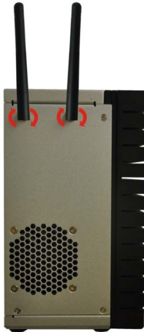
Figure 3-9: Wi-Fi Antenna Installation
