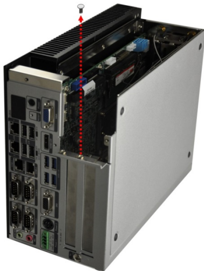
Figure 3-32: Remove Expansion Slot Bracket
