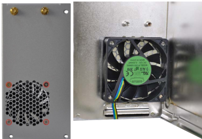
Figure 3-8: System Fan Installation (P/N: 32128-002900-100-RS)
