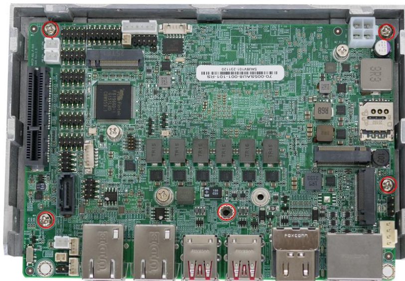
Figure 4-3: Heat Sink Retention Screws
