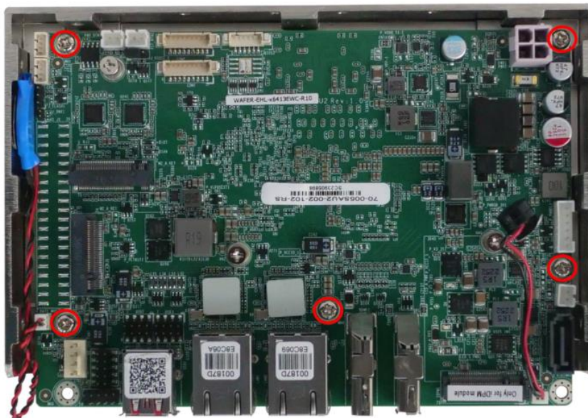
Figure 4-3: Heat Sink Retention Screws
