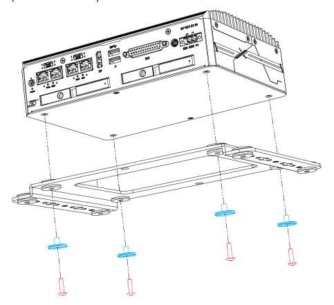
3. Make sure you secure the system on a flat surface. The illustration shows only the anti-vibration mount being secured.
