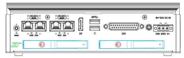
The system supports two external 2.5" HDD/ SSD via front-accessible trays. Designed for easy access, the HDD trays are secured by a lock (indicated in red) and together. There is a disk connector insertion orientation (indicated in green) to avoid damaging the connectors during installation.
