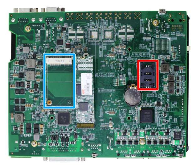
This mini-PCle socket works (indicated in **blue**) in cooperation with the SIM slot (indicated in **red**). By installing a mini-PCle module, you can add additional features to your system such as WIFI, GPS, CAN bus, analog frame grabber, etc. You can also install a 3G/4G module and SIM card for internet via your service provider's 3G/4G network.
