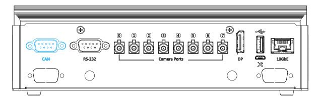
CAN bus is a robust industrial bus with a pair of differential signals and is commonly used in various industrial and in-vehicles applications. The system is equipped with a CAN bus DB9 port that is compatible with both industrial and in-vehicle applications. The CAN bus port supports CAN2.0A and CAN2.0B up to 1Mbps.
