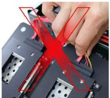
**DO NOT** push the connector while holding the cable
