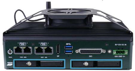
The system has two front accessible 2.5" HDD/ SSD trays that can accept 2.5" HDD/ SSD up to 9.5mm. To install a HDD/ SSD into the tray, please refer to the following instructions.
