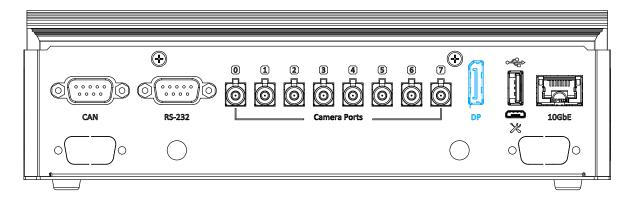
The system has a DisplayPort (DP) output which is a digital display interface that mainly connect video source and carry audio to a display device. Please use cable length within 1.8 meters when connecting a DP, the port can deliver up to 4K UHD (3840 x 2160 @ 30Hz) in resolution.
