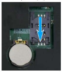
5. Insert the SIM card and secure the holder by sliding the holder away from the battery.
