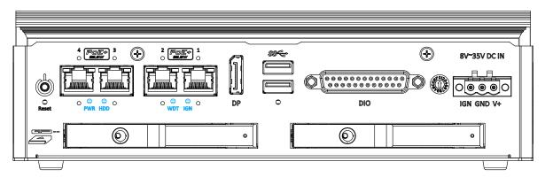
There are four LED indicators on the front panel: PWR, HDD and IGN. The descriptions of these four LEDs are listed in the following table.
