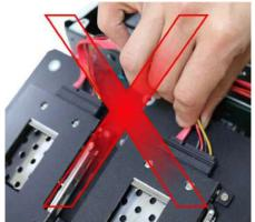
Pull to disconnect by placing fingers on the connector
