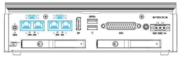
The Gigabit Power over Ethernet (PoE) port supply power and data on a standard CAT-5/CAT-6 Ethernet cable. Acting as a PSE (Power Sourcing Equipment), compliant with IEEE 802.3at, each port delivers up to 25W to a Powered Device (PD). PoE automatically detects and determine if the connected device is PoE PD or not before supplying power, making it compatible with standard Ethernet devices as well. There are screw-lock holes (indicated in red) for each port to ensure cables are tightly secured
