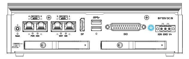
The ignition power control switch features multiple modes for pre and post ignition settings. Please refer to the section <u>Ignition Power Control</u> for details.
