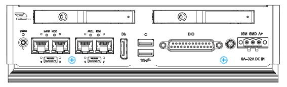
4. Secure the two screws indicated on the rear panel.
