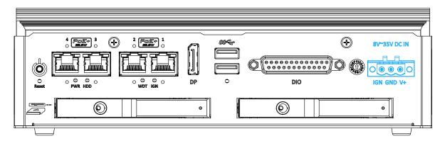
The system allows an 8 to 35V DC power input from via a 3-pin pluggable terminal block. The screw clamping mechanism is a reliable way to wire DC power. In addition to DC power, this terminal block also accepts ignition signal input (IGN).
