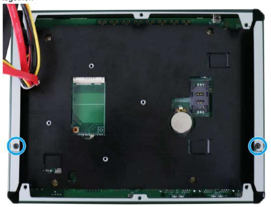
3. Secure the two screws indicated on the front panel.
