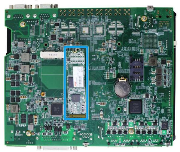
The system has an M.2 2280 slot (M key PCIe Gen3 x2) to install an NVMe SSD for the ultimate disk read/ write performance. An NVMe SSD offers significantly more disk read/ write speed performances over 2.5" SSDs.
