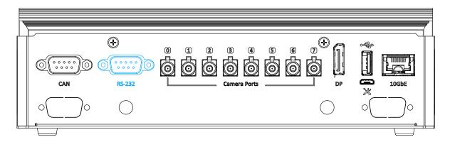
The system has a RS-232 COM port for communicating with external devices. The port can be located on the rear panel via 9-pin D-Sub male connectors.
