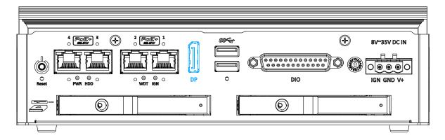
The system has a DisplayPort (DP) output which is a digital display interface that mainly connect video source and carry audio to a display device. When connecting a DP, it can deliver up to 4K UHD (3840 x 2160 @ 30Hz) in resolution. The system is designed to support active DP adapter/ cable from NVIDIA's recommended display adapters. You may refer to NVIDIA's page to find more information
