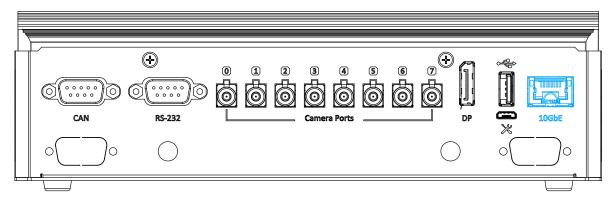
Utilizing Intel's X550-AT2 controller, the RJ45 10GBAST-T connector offers up to 10Gb bandwidth throughput over a maximum distance of 100 meters using Cat 6a or 55 meters using Cat 6 cables. It is ideal as a camera hub to deliver real-time image or video to other computers.
