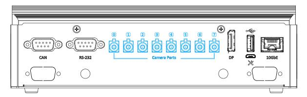
The NRU-110V system features eight FAKRA Z male camera connection ports that support automotive camera sensors. Coupled with the unique onboard trigger system, it can simultaneously capture images from eight GMSL cameras within millisecond channel-to-channel skew.
