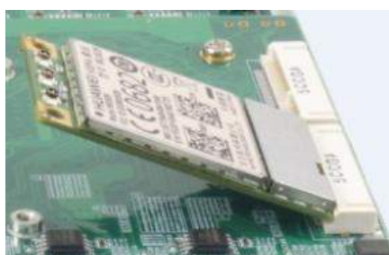
45 degree insertion angle
