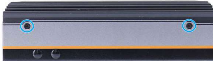
Right side chassis screws securing the heatsink
