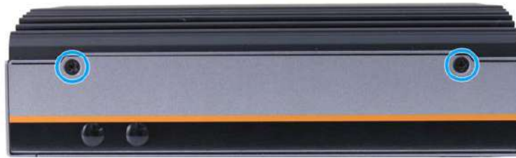
Left side chassis screws securing the heatsink
