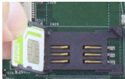
Insert Mini-SIM card with pins facing up
