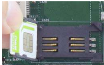
Insert Mini-SIM card with pins facing up
