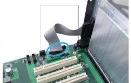
Disconnect 4-pin fan connector
