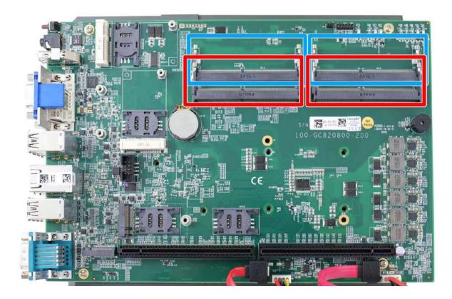
The system motherboard supports four 260-pin SODIMM socket for installing ECC/ non-ECC DDR4 memory module up to 128GB. Each slot supports single module DDR4 2133MHz SODIMM up to 32GB capacity.
