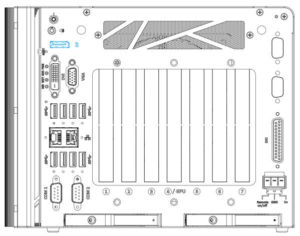
The DisplayPort (DP) output is a digital display interface that mainly connect video source and carry audio to a display device. When connecting a DP, it can deliver up to 4K UHD (4096 x 2304) in resolution. The system is designed to support passive DP adapter/ cable. You can connect to other display devices using DP-to-HDMI cable or DP-to-DVI cable.
