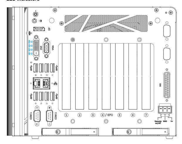
There are four LED indicators on the I/O panel: IGN, WDT, HDD and PWR. The descriptions of these four LED are listed in the following table.
