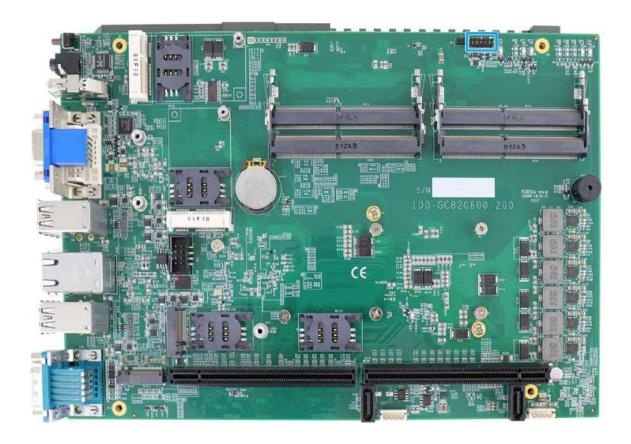
For an application which places the system inside a cabinet, it's useful to have an external system status LED indicators. The system provides a 2x6, 2.0mm pitch pin header to output system status such as power, HDD, watchdog timer, and control system on/ off remotely.
