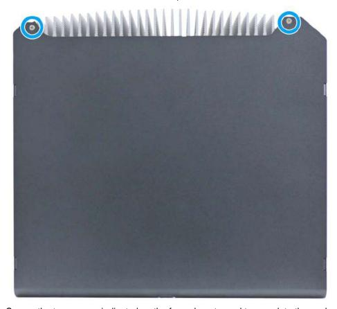
5. Secure the two screws indicated on the fan exhaust panel to complete the enclosure installation process.
