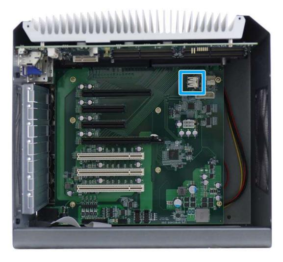
The system's daughter board has an internal USB2.0 port on the PCBA. You can utilize this USB port to connect a USB protection dongle inside the chassis of the system.
