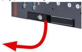
3. Insert the HDD/ SSD (with labels facing up) and the SATA connector end towards the slot, insert it 3/4 of way in and use the lever to fully push the HDD/ SSD into the slot. You should hear a click sound to ensure the HDD/ SSD is properly inserted and engaged.
