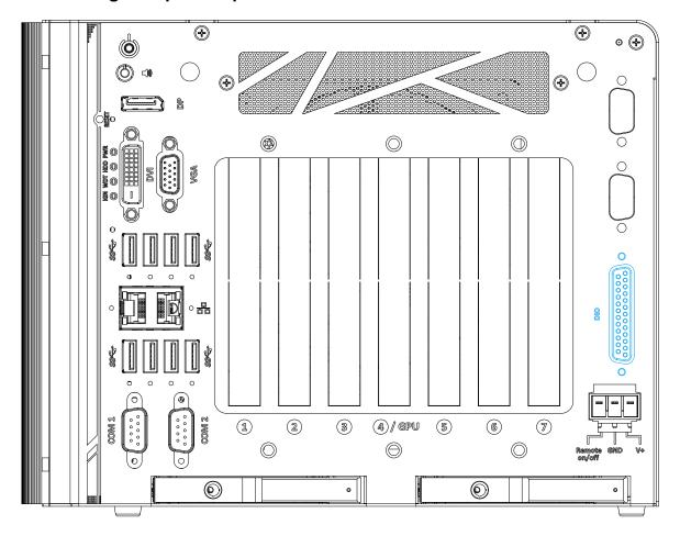
The system provides 8x isolated digital input channels and 8x isolated digital output channels.
