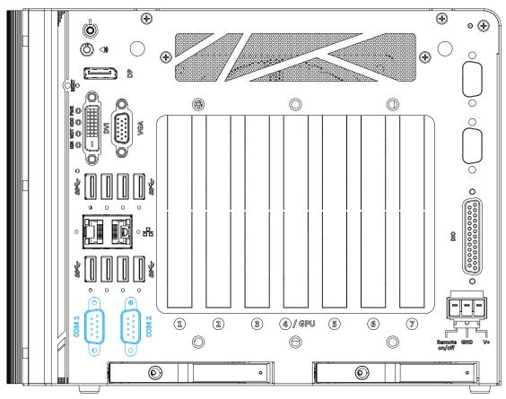
The two COM ports are implemented using industrial-grade ITE8786 Super IO chip (-40 to 85°C) and provide up to 115200 bps baud rate. COM1 and COM2 are software-configurable RS-232/422/485 ports. The operation mode of COM1 and COM2 can be set in BIOS setup utility. The following table describes the pin definition of COM ports.
