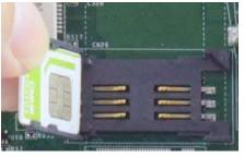
Insert Mini-SIM card with pins facing up
