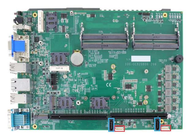
The system provides two SATA ports which support Gen3, 6 Gb/s SATA signals. Each SATA port (indicated in blue) features a 7-pin SATA connector and a 4-pin power connector.
