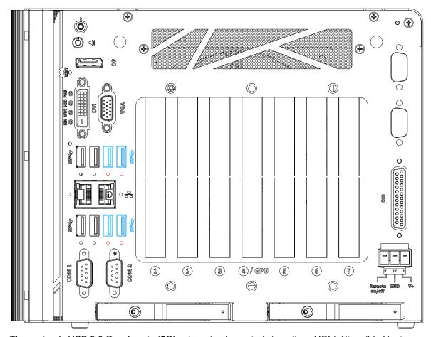
The system's USB 3.0 Gen 1 ports (5Gbps) are implemented via native xHCI (eXtensible Host Controller Interface) controller and are backward compatible with USB 2.0, USB 1.1 and USB 1.0 devices. Legacy USB is also supported so you can use USB keyboard/mouse in DOS environment. There are also screw-lock openings (indicated in red) for each USB port. xHCI driver is supported natively in Windows 10, therefore you do not need to install xHCI driver in prior to utilize USB functions.
