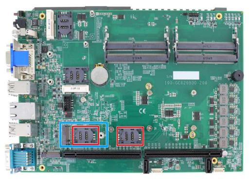
3. Before installing the mPCle module, you need to insert the Mini-SIM card. Slide the SIM slot holder and lift the SIM card holder. Insert the Mini-SIM card (pins facing up), shut the SIM holder and slide it to lock the SIM card in-place.
