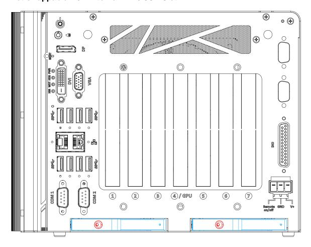
The system supports external 2.5" HDD/ SSD hot-swappable slot(s). Designed for easy access, the HDD/ SSD slot is secured by a lock (indicated in **red**) and it supports RAID modes 0/ 1 configuration for OS installation. To set up RAID, please refer to RAID Volume Configuration section for details.
