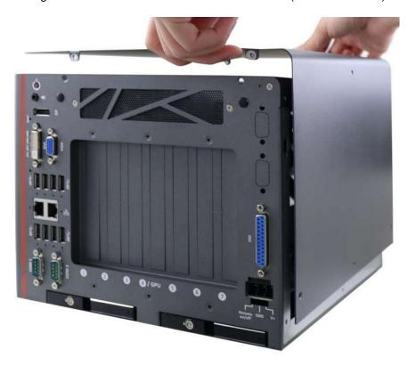
Place L-shape side panel onto the enclosure
