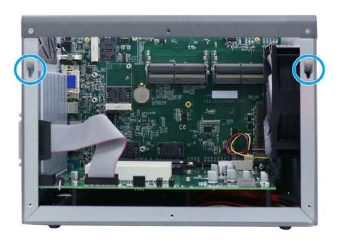
Slide-and-lock into the indicate hinges
