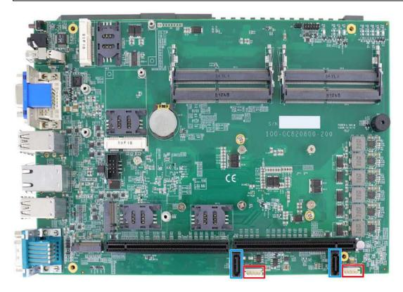
The system has two SATA ports (indicated in **blue**) and two four pin power connectors (indicated in **red**). The SATA and power cables should already be connected on the motherboard so users only need to install the HDD/ SSD. Please refer to the following instructions on how to install 2.5" SATA HDD/SSD.
