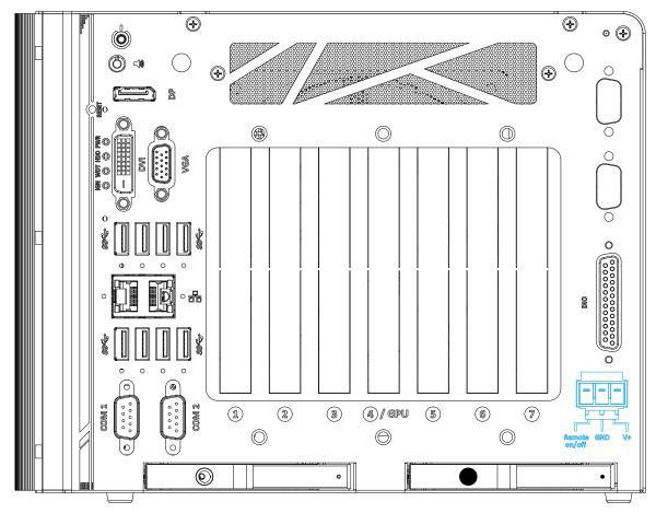
The system accepts a wide range of DC power input from 8 to 35V via a 3-pin pluggable terminal block, which is fit for field usage where DC power is usually provided. The 3-pin terminal block also offers "Remote On/ Off" that allows for external switch extension. It is useful when the system is placed in a cabinet or a not easily accessed location. You may connect an external status LED (20mA) indicator by connecting to PWR LED and GND.
