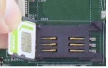
Insert Mini-SIM card with pins facing up
