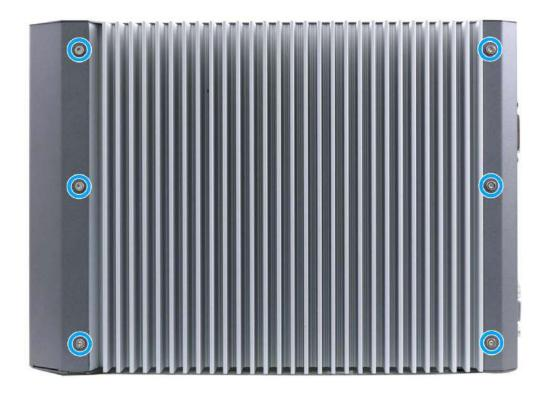
10. Remove the screws indicated in blue to separate the motherboard from the heatsink. If your system already has a CPU installed, you will also need to remove screws in locations indicated in red before separating the motherboard from the heatsink.
