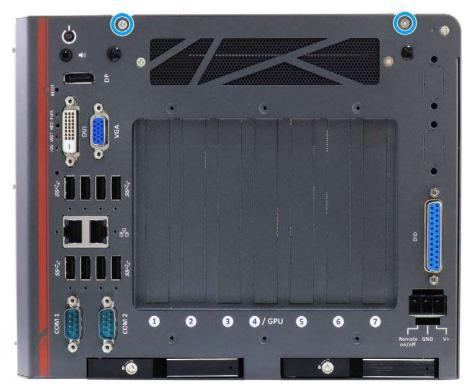
2. Remove the screws indicated on the side panel.
