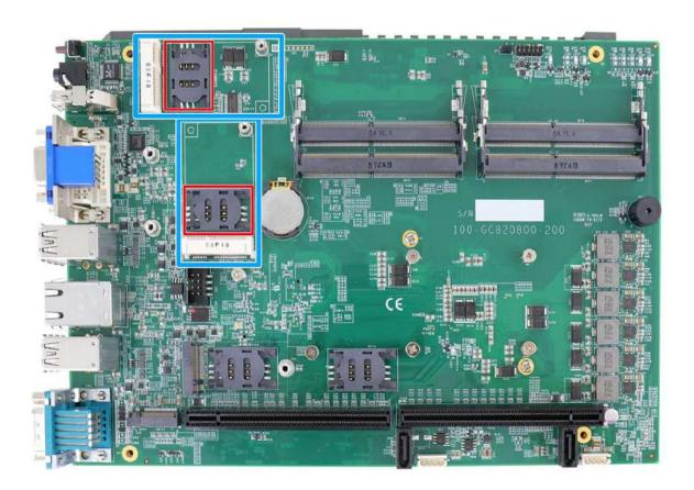
For wireless (WIFI/ 3G/ 4G) communication, multiple SMA antenna apertures (indicated in blue) can be located on the front and rear panel.
