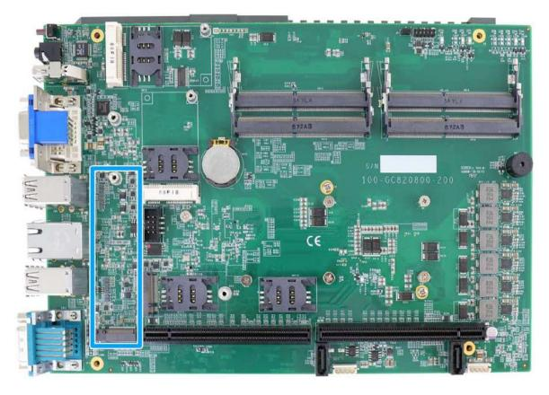
The system has anx4 PCIe M.2 2280 slot (also in compliance with SATA signal) for you to install an NVMe SSD for the ultimate performance or an Intel<sup>®</sup> Optane<sup>TM</sup> memory to accelerate the read/ write performances of traditional hard disk drive. An NVMe SSD offers exceptional performance over 2.5" SSDs while Intel<sup>®</sup> Optane<sup>TM</sup> memory can dramatically boost your traditional hard disk drives' read/ write performances.
