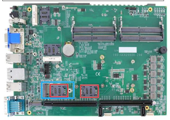
The system has anM.2 2242 slot (indicated in **blue**) that works with dual SIM slots (4G + 3G) indicated in **red**. By installing a 3G or 4G M.2 module and SIM card, you can access the internet via the provider's network.
