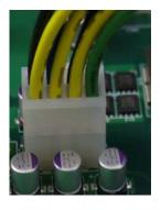
6-pin power connector on extension board
