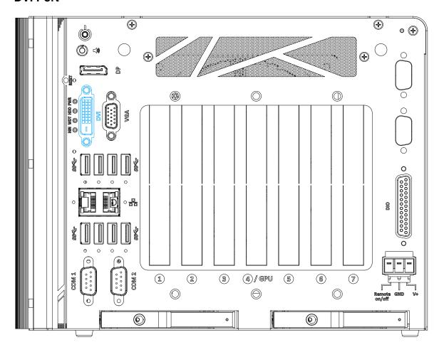
DVI-D transmits graphics data in digital format and therefore can deliver better image quality at high resolution. The DVI connector on the front panel can either output DVI signals or other digital signals (via an adapter/ cable) depending on the display device connected. It supports resolutions up to 1920x1200@60Hz.
