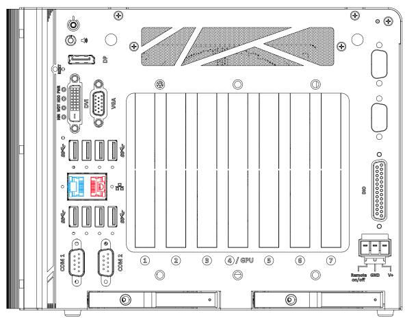
The system offers 2 GbE ports on its I/O panel. The GbE ports are marked in blue/ red and are implemented with Intel® I219-LM/ Intel® I210-IT controllers, respectively. Each port has one dedicated PCI Express link for maximum performance. When an Ethernet connection is established, the LED indicators on the RJ45 connector represents the following connection statuses:
