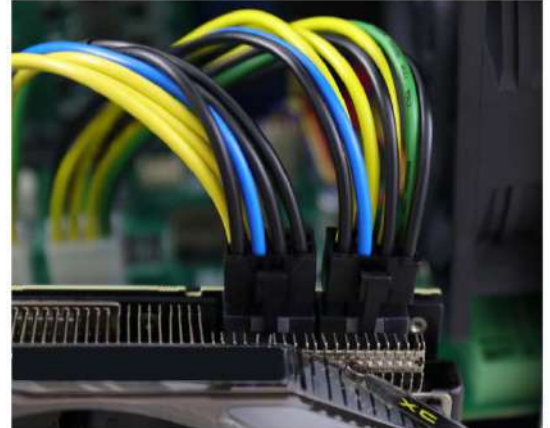
6 or 8/ 8-pin power connector on graphics card
