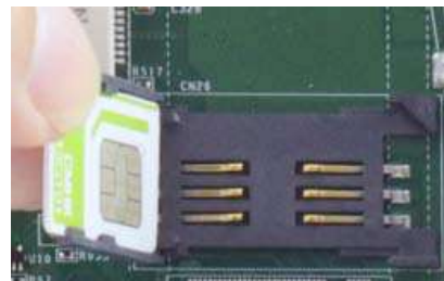
Insert Mini-SIM card with pins facing up
