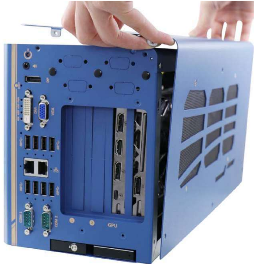
Place L-shape side panel onto the enclosure
