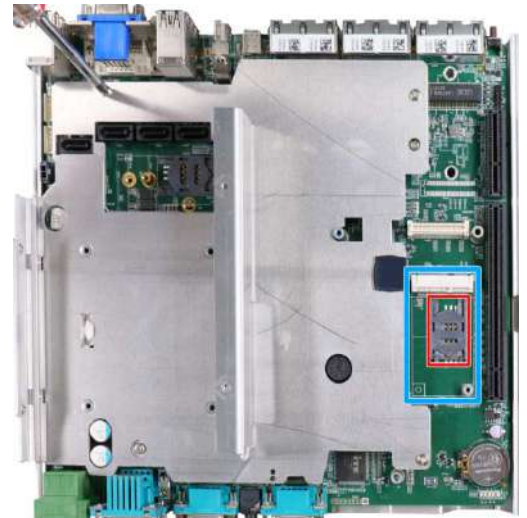
mini-PCIe slot on motherboard (underneath MeziO™ card)
