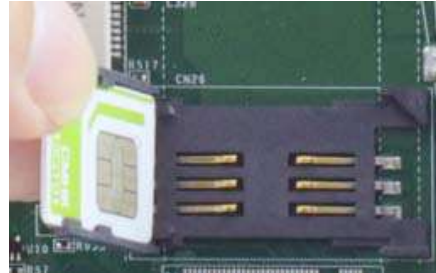
Insert Mini-SIM card with pins facing up
