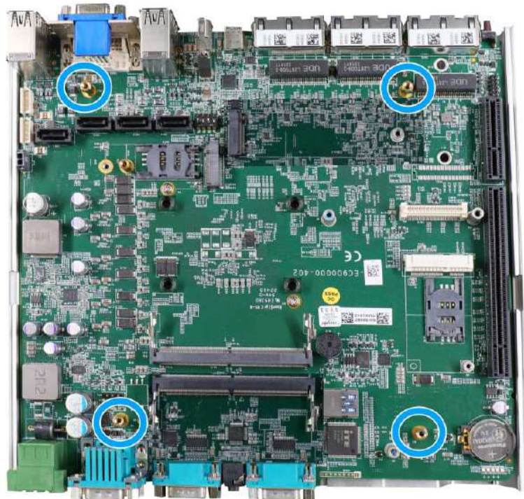
Secure motherboard with four screws
