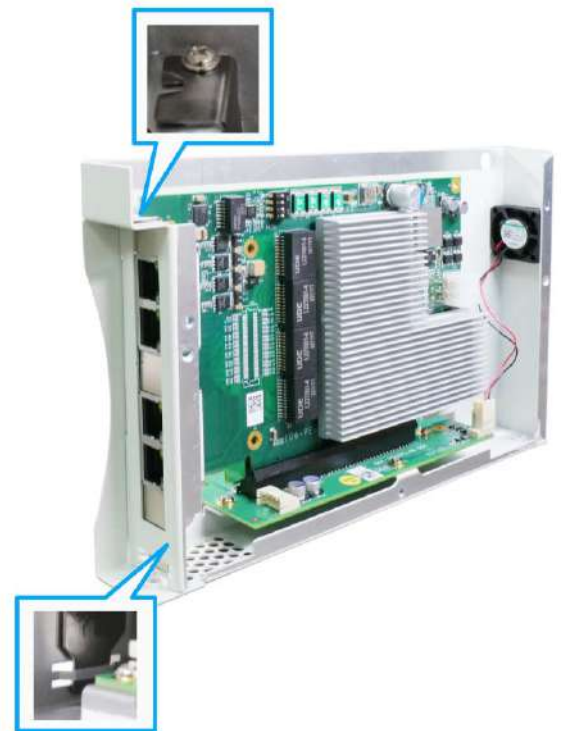
Make sure the card is inserted into the notch and secured with a screw
