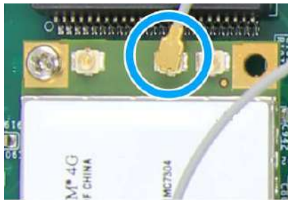
Clip on IPEX-to-SMA cable
