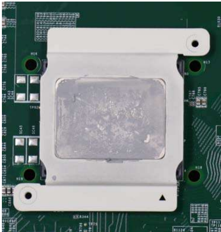
CPU retention bracket (holder)
