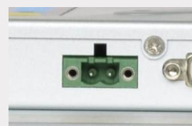
Phoenix terminal using fastening type power connector
